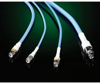
PhaseTrack<sup>®</sup> cable assemblies are designed for applications demanding minimal phase change over temperature. All PhaseTrack cables use proprietary TF4<sup>™</sup> dielectric that does not have the abrupt shift in the phase that occurs with solid or tape wrapped PTFE based products under normal room ambient temperature conditions.
